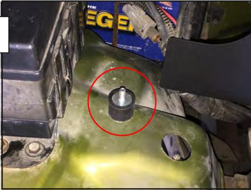
Install the intake tube mount through the fender using the supplied mount, washer and flange nut.
