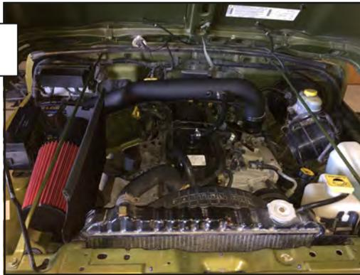
Install the air filter using the supplied clamp.
