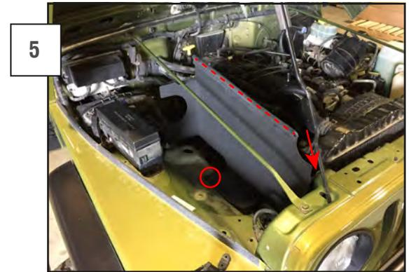
Install the heat shield using the supplied M8 bolt, washers, and nut. Reinstall the factory bolt through the heat shield mounting hole. Install the supplied weather stripping across the top end of the heat shield.
