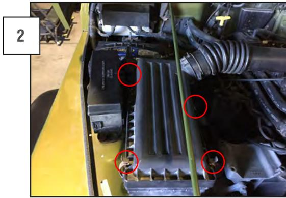
Unclip the (4) clips to remove the top of the air box.
