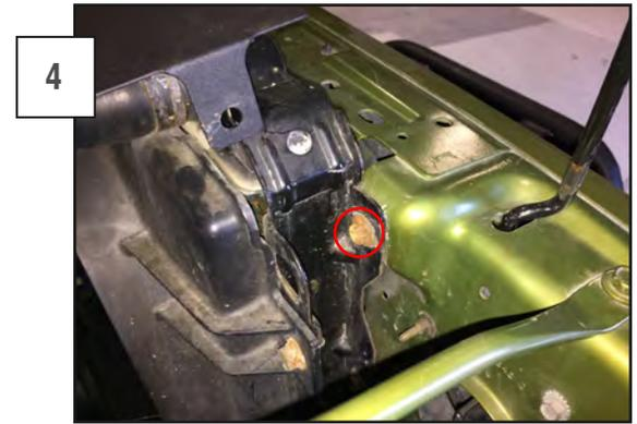
Remove the bolt holding the radiator bracket to the radiator support.
