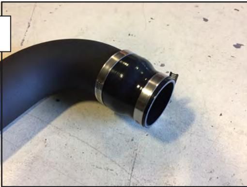
Install the silicone coupler and clamps to the throttle body side of the intake tube. Loosely install the intake tube to the throttle body. \*\*Note: 97-04 vehicles install the plug into the intake pipe. 05-06 vehicles install the Rubber grommet into the intake pipe for the IAT Sensor. Fasten the intake tube to the mount using the supplied washer, and flange nut. Then tighten the hose clamps on the throttle body.
