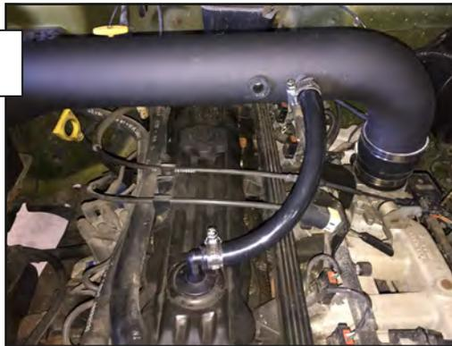
Install the supplied vacuum hose, trim for best fit. Secure using the supplied hose clamps.
