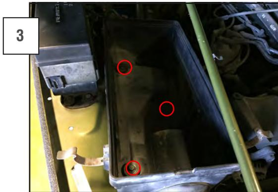
Remove the air box by removing the (3) bolts securing it to the vehicle.
