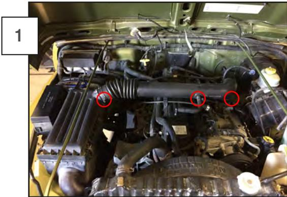
Remove the factory intake tube by loosening the hose clamp on the throttle body and air box. Remove the PCV line from the intake pipe.
