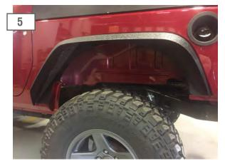
Install the M6x1.00 25mm bolts with the supplied washer and lock washer on all mounting locations containing rivnuts.
