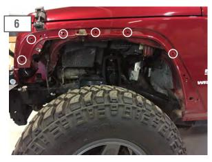
Drill the circled (6) holes above to 25/64". Rivnuts will be installed in step 6.
