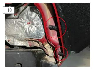
Re-install the fender using the supplied hardware on all mounting location containing rivnuts. Install the supplied spacers between the inner and outer fenders. The longer spacer uses an M8x1.25 115mm bolt, flat washer, lock washer, and nut. The short spacer uses an M8x1.25 65mm bolt, flat washer, lock washer, and nut.
