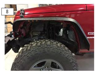
Test fit the fender by installing the M6x1.00 25mm bolts with the supplied washer, and lock washer on all mounting locations containing rivnuts. (4) Addition holes will need to be drilled in step 8.
