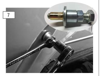
Rivnuts provide solid mounting point when there is no access behind the mounting surface. Insert the rivnut into the pre-drilled hole. Thread the rivnut tool onto the rivnut. Using a 16mm wrench, hold the nut in place while turning the head of the bolt with a 17mm ratchet. Tightening the bolt will clamp the rivnut against the sheet metal. \*\*Note: Do not over tighten the rivnut. Doing so can pull the threads out of the insert.
