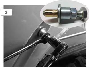
Thread the rivnut tool onto the rivnut. Using a 16mm wrench, hold the nut in place while turning the head of the bolt with a 17mm ratchet. Tightening the bolt will clamp the rivnut against the sheet metal. \*\*Note: Do not over tighten the rivnut. Doing so can pull the threads out of the insert.
