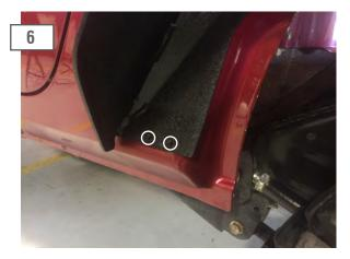
Install the (2) self-tapping screws once the fender has been fully installed.
