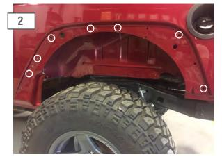
Install the supplied rivnuts in the (7) holes circled above. Begin by drilling the rivnut holes to 25/64".
