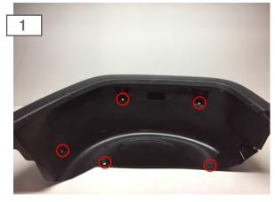
Using a flat head screw driver, remove the (5) push clips holding the rear fender liner to the vehicle. Then firmly pull the stock fender away from the vehicle moving from front to back. The factory clips will most likely break, the clips will not be reused.
