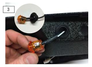
Slide the LED grommet off the back of the lights as shown. Feed the light's plug through the hole in the fender. Press the grommet into the fender, then press the light into the grommet. \*\*Note: There is a "Top" marked on the light.
