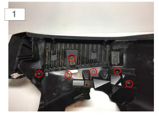
Begin by removing the factory fender liners, there are (5) 10mm bolts. Remove the factory marker light harness from the light. Remove the factory fender by firmly pulling it away from the vehicle. Start from the front of the fender and work towards the rear. The factory clips will most likely break, the clips will not be reused.
