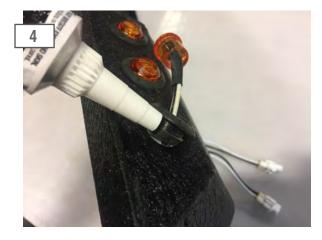
The rubber light grommet is a press fit. If there is play in the grommet after and the light is installed apply a small amount of silicone adhesive to the grove on the back side of the grommet.
