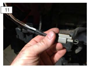
Plug the LED main harness into the vehicles marker light plug. Secure any extra wire out of the way using the included zip ties.
