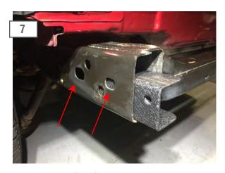
Next, slide the (2) L-Shaped mounting brackets into the frame rails with the nut backing up to the factory holes in the frame.
