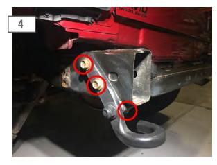
Remove the (3) bolts securing the tow hook to the driver side frame rail.
