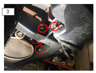
Remove the (4) 15mm bolts on the outside of each frame rail. Then remove the (4)15mm bolts securing the plastic bumper to the frame. Remove the bumper from the vehicle.
