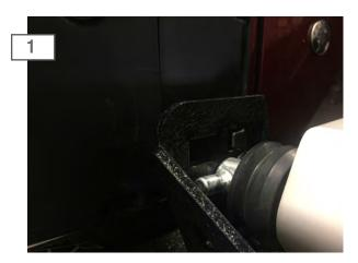
If the tire carrier arm sits to low on the tire carrier latch, adjustment of the tire carrier post will be required.
