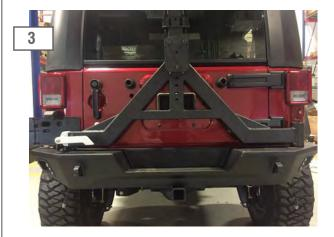
Lift the carrier arm until the latch is aligned. \*\*Note: Depending on the weight of the spare tire, it may be necessary to align the carrier arm slightly above the latch opening. The weight of the tire will create proper alignment. Once aligned re-torque the carrier post mounting bolts to 64lb ft. Install the spare tire and test latch alignment. Adjust the post mount as needed.
