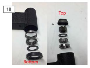
Install the larger bearing and race into the bottom of the tire carrier, and the smaller bearing and race on the top of the tire carrier. Make sure to pack the bearing with grease before installation. Then use the small washer for the top and the larger washer for the bottom. Install the seal on the bottom of the tire carrier. Also use a small amount of grease for the seal.
