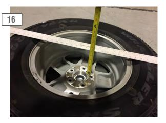
Measure the backspacing of your wheel and tire by placing a straight edge across the tire. Measure from the mounting hub to the straight edge. Subtract a half inch from the previous measurement, and set the carrier to the new measurement. This ensures the tire sits tight against the carrier.
