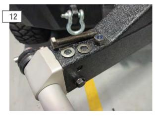
Install the carrier latch handle using (2) M10 x 1.5 x 65 bolts, washers, and lock nuts.
