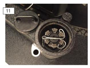
Install the tire carrier. Be sure to add a little extra grease for good lubrication. Use the supplied castle nut and cotter pin and a 35mm socket to seat the tire carrier to the tire carrier shaft. Then install the dust cover and small phillips set screw.
