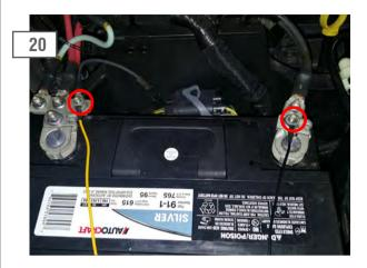
Optional Flood Light Wiring: Install the yellow 12+ volt wire to the positive battery terminal. Connect the black ground wire to the negative battery terminal. Zip tie the excess wiring away from any hot/and or moving parts.
