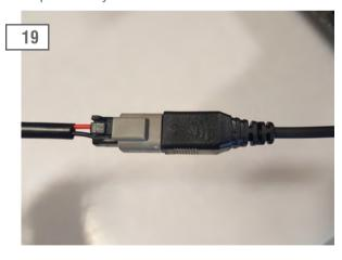
**Optional Flood Light Wiring:** Connect the (2) LED Flood lights into the supplied harness. Zip tie the excess wiring away from any hot/and or moving parts.
