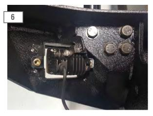
Install the optional Flood lights using the hardware provided in the light packaging. If choosing not to use the LED lighting. The bumper will include bolt on mesh covers. Secure the cover to the bumper using the provide (2) M6x1.0 20mm bolt and flat washer.
