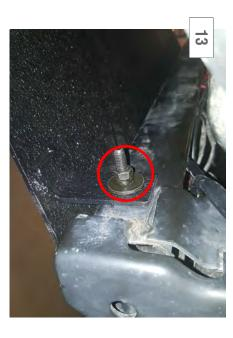
supplied (2) M8 x 1.25 x 40mm hex head bolts, Install the skid plate to the chassis using the lock washers, large washers, and nuts. Optional Skid Plate Installation:
