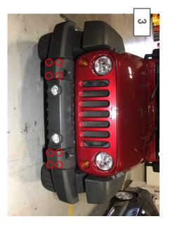
From under the vehicle, access and remove the (8) 18mm nuts securing the factory bumper to the vehicle.
