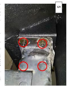
Install the bumper by using the (4) M10 nuts, (4) M10 x 25mm bolts, (8) lock washers, and (8) flat washers to the vehicle. Torque to 40 lb ft.
