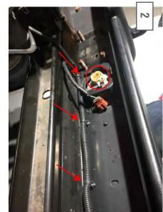
From under the vehicle, remove the factory fog light connectors and free the fog light wiring loom from the bumper.
