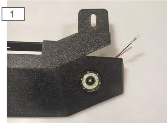
Install the (4) LED Rock lights to each of the rock sliders using the M8 Bolt/washer.
