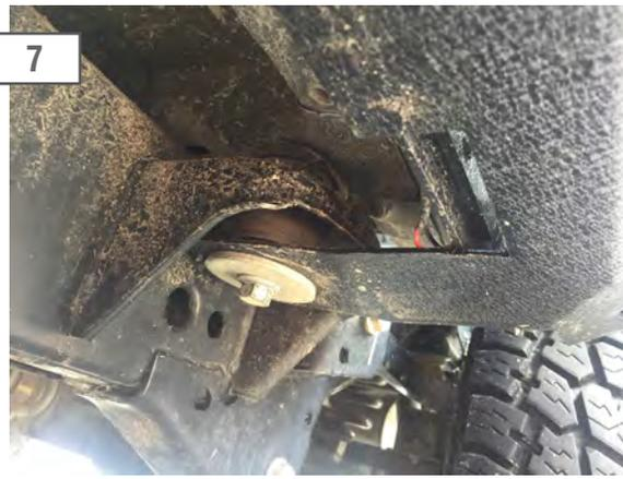
Once the Rock Sliders are tight to the pinch welds, tighten the body mount bolt to 80 lb. ft. Remove the nut plate handle by bending it back and forth until it breaks off.
