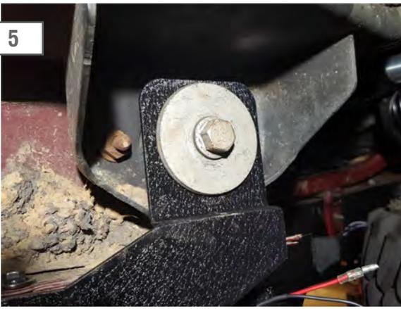
Loosely install the rock sliders using the factory 18mm bolts.
