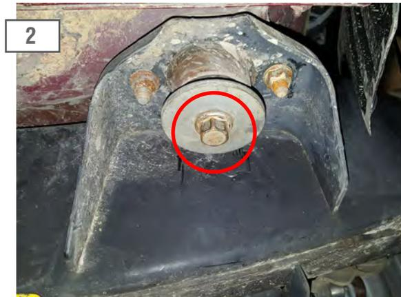
From under the vehicle access and remove the 18mm body mount bolts. (4) Bolts on 2 door, and (6) Bolts on 4 door vehicles. \*\*NOTE Factory hardware will be reused.
