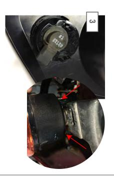
the turn signal tabs to align correctly. cause the grille to stick out. It may be necessary to the lower headlight bucket tab. Failure to do so will installed the tabs on the turn signal need to straddle the outer edge of the grille. When the grille is the turn signal so that the connector points towards rotate the signals slightly once installed in order for Transfer the turn signals to the new grille. Position
