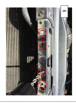
Using a 11/32" drill bit, enlarge the (4) factory holes on the radiator support to accept the supplied rivnuts. Rivnuts provide solid mounting point when there is no access behind the mounting surface.
