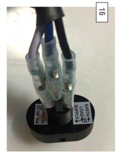
Connect the wiring to the switch as seen above. Black is ground, White is supply, and blue is load.
