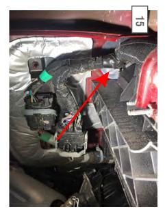
Feed the switch wiring through a firewall grommet into to the interior of the vehicle. Mount the switch as desired.
