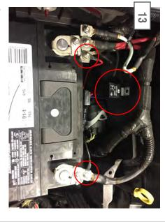
Connect the red ring terminal to the positive (+) battery terminal. Connect the Black ring terminal to the negative (-) battery terminal. Secure the relay out of the way.
