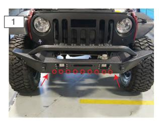
Identify the skid plate mounting locations as shown above.
