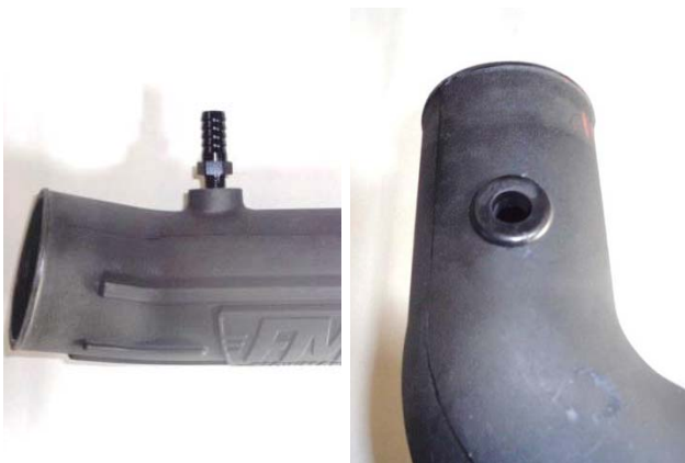
15. Apply 2 wraps of nylon thread tape to threads of barbed PCV fitting (18), and install fitting in intake tube (19). Install rubber grommet (16) in intake tube.
