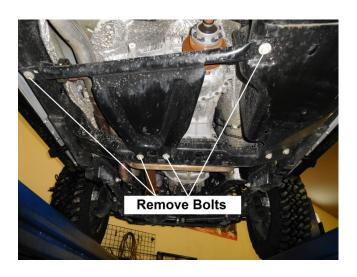
7) Support the center of the fuel tank with a jack or a stand. Use a ratchet and an18mm socket to remove Qty. 5 bolts of 7 that hold up the fuel tank. Then only loosen the last two bolts in the back. Lower the jack or stand to allow the front of the fuel tank to drop down to expose the transmission crossmember bolts on the passenger side.
