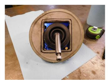
12) Use a ratchet with a T30 torx socket to unbolt and remove the stock shifter.
