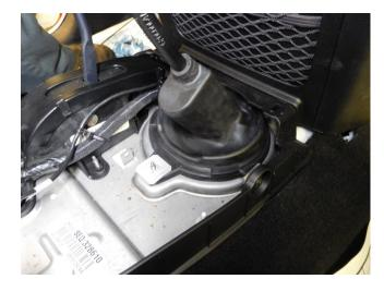
19) Reinstall the center console and press the factory knob onto the shifter and transfer case stick.
