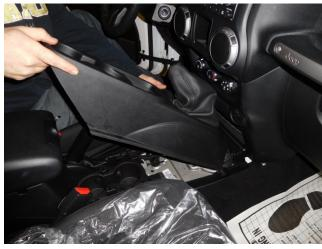
3) Unscrew the square secure plate holding the rubber boot over the shifter. Then remove the rubber boot.
