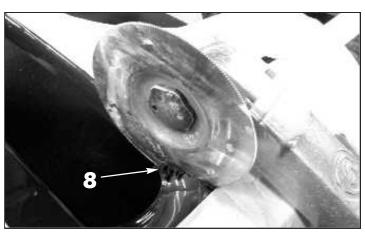
**8.** Use a jig or vibrating saw to cut through the sides of the grille where marked in the previous steps.
