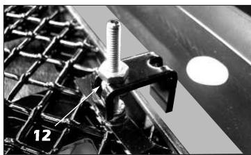
**12.** Align the U-shaped grille retainers across the top of the grille and install a #8-32 ESNA half nut and tighten until the grille surround is flush with the factory grille.
