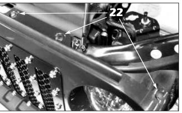
**22.** Reinstall the factory push pins across the top edge (driver side shown) and close the hood to finish the installation.
