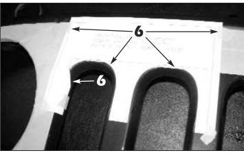
**6.** Cut out and align the upper grille cutting template and tape it in place as shown. Use a sharpie or grease pencil to mark the side of the grille where the template folds down on the side. Untape the template, turn it over, align it on the opposite side and tape it into place and mark the side of the grille.
