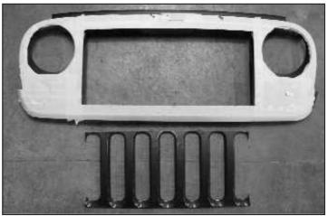
10. The finished cut should look like this. Factory grille center section is not reused. Remove the protective masking tape once the cutting is finished.
