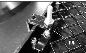
**14.** Align the U-shaped grille retainers onto each side of the grille and install a #8-32 ESNA half nut and tighten until the grille surround is flush with the factory grille.
