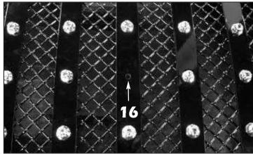
**16.** If the grille will use the supplied emblem plate, remove the center 12 point stud from the grille using a small punch and mallet from the reverse side.
