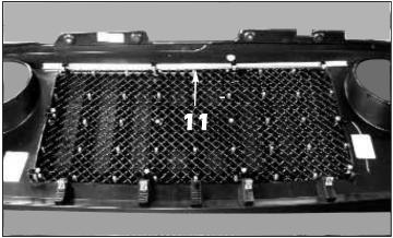
**11.** Align the cut factory grille over the E&G E-Power mesh grille as shown. Align the supplied upper grille reinforcement across the top edge of the inside of the factory grille prior to U-shaped grille retainer installation.
