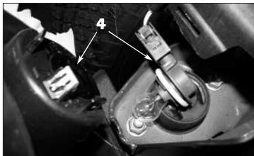
**4.** Carefully rotate the turn signal bulbs to remove them from the lamp sockets attached to the factory grille.
