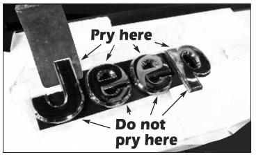
**5.** If using a tucking tool to remove the Jeep lettering, do so from the top down. Do not work from the bottom up or you will damage the paint at the tops of the letters. You can also use fishing line to cut through the factory double faced tape.
