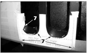
7. Cut out and align the lower grille cutting template and tape it in place as shown. Use a sharpie or grease pencil to mark the side of the grille where the template folds down on the side. Untape the template, turn it over, align it on the opposite side and tape it into place and mark the side of the grille.
