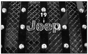
19. Peel off the double faced tape backing, align the Jeep lettering onto the emblem mounting plate and install it onto the E-Power grille using the large black plastic washers between the emblem plate and the mesh. You might have to clip a mesh wire in order to center the emblem.
