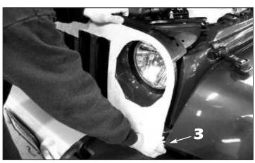
3. Hold the top edge of the grille and give the grille several quick tugs across the bottom edge to unclip it from the support. Do not pull the grille too far out, the turn signal bulbs are attached to the back of the grille.
