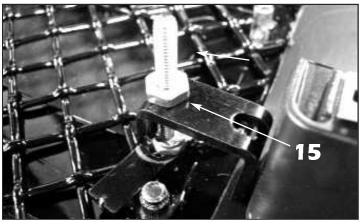
**15**. Align the U-shaped grille retainers across the bottom of the grille and install a #8-32 ESNA half nut and tighten until the grille surround is flush with the factory grille.
