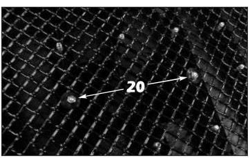
**20.** Turn the grille over and secure the emblem assembly using the supplied large black plastic washers and the #8-32 ESNA half nuts.
