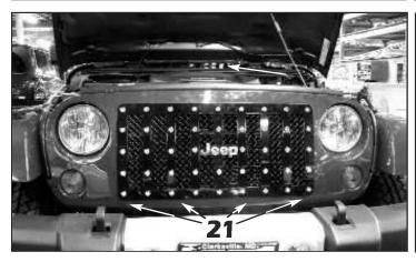
**21.** Align the assembled grille back onto the vehicle and clip the lower edge into place.
