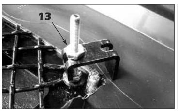
**13.** Align the U-shaped grille retainers into the lower corners of the grille and install a #8-32 ESNA half nut and tighten until the grille surround is flush with the factory grille.
