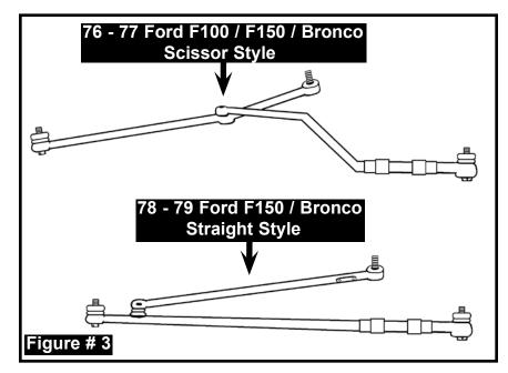
76-77 Ford F100 / F150 & Bronco. The drag link & tie rod assembly will require changing to the "Straight Style" steering found on the 78-79 Ford F150 & Bronco in order to install a drop pitman arm. (See Figure # 3)
