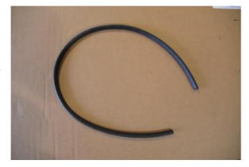
Cut the strip to fit the length of the front edge on both fenders and stick on fender before installing bumper.
