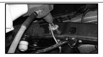
Working on the driver side, carefully remove the ABS line clip from the bottom of the frame rail. Repeat procedure on the passenger side.
