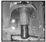
8. Locate the new front coil springs. Working on the driver side, install the new coil spring into the OE location. Carefully raise up on the hydraulic floor jack until the coil spring seats properly into the vehicle. Repeat procedure on the passenger side.
