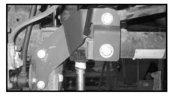
27. Locate the new rear sway bar end links. Locate (8) poly Repeat procedure on the passenger side. bushings and (4) S10026 sleeves from hardware bag 43000NB1. Install the new bushings and sleeves into the new end links. Special note: Make sure to use a fair amount of lithium or moly base grease before installing the new bushings and sleeves into the end links. This will increase the life of the bushing as well as help prevent squeaking.
