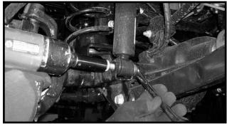
6. Carefully lower down on both hydraulic floor jacks at the same time allowing enough room for the coil springs to be
