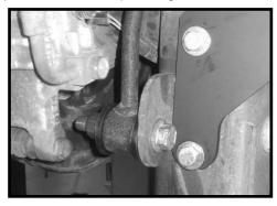
29. Locate (2) 1/2" x 2 1/2" bolts, (4) 7/16" USS flat washers and (2) 1/2" unitorque nuts from hardware bag 43000NB. Working on the driver side, install the new end link to the inside of the sway bar and secure using the new 1/2" hard-
