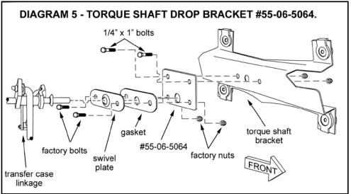
Attach the swivel plate and gasket to the Superlift torque shaft bracket (#55-06-5064) using the supplied factory bolts and nuts (18).
