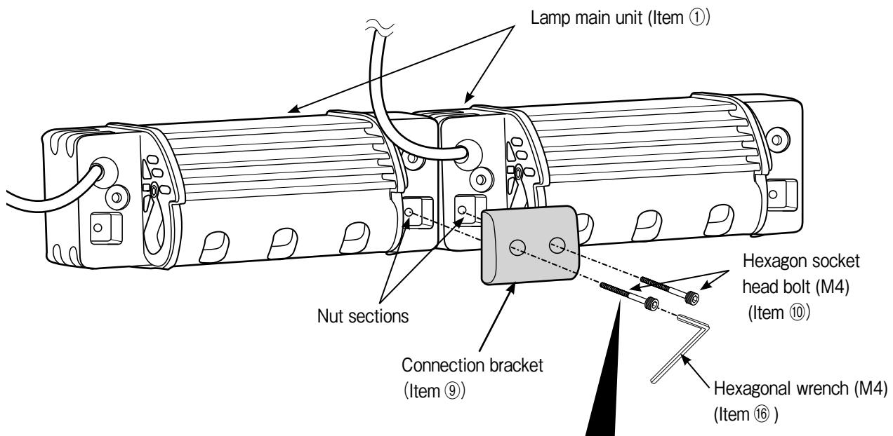
Tightening torque : 2.2ft/lbs (3N·m)
