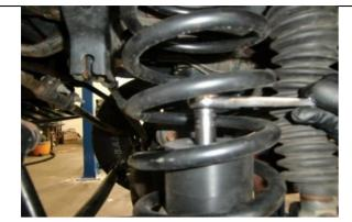
Secure bump stop extensions to axle with provided hardware.
