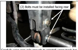
Carefully raise rear axle enough to reinstall upper track bar.
