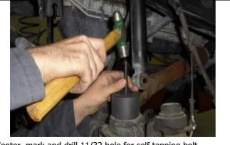
Center, mark and drill 11/32 hole for self tapping bolt.
