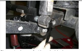
Disconnect and remove front lower shock hardware.
