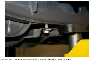
Remove (2) front transfer case skid plate bolts.
