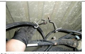
At the rear, remove center brake line nuts under body.
