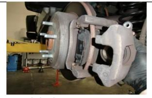
Remove rear brake calipers.
