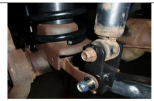
Raise axle and reinstall OE front shocks and torque to spec.
