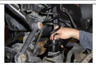
Install new springs/bump stops extensions simultaneously.
