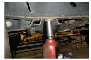
Reinstall front transfer case skid plate bolts.
