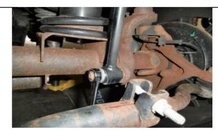
Attach the stock rear sway bar end links to the front sway
