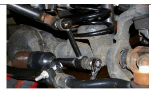
Remove dr./pass. lower front sway bar end links. These will be replaced with the stock rear end links later.
