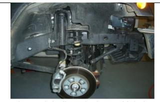
Securely raise vehicle off ground and remove (4)wheels
