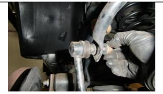
Disconnect and remove rear sway bar end links. Save these links as they will be used on the front sway bar.
