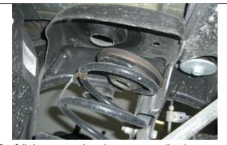
Carefully lower rear axle and remove rear coil springs.
