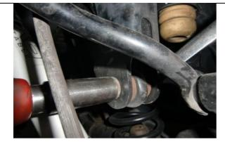
Slightly lift rear axle and remove upper track bar bolt.
