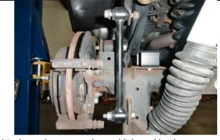
Attach new longer sway bar end links and hardware.
