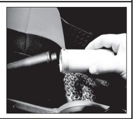
Step 2. Tighten both Allen head set screws. Do not overtighten. Test emergency brake handle to ensure proper function before operating vehicle.
