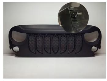
**Step 3\\**Press on the (6) supplied retaining clips. Using the factory grille as a reference, apply the supplied weather stripping across the top of the grille.
