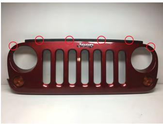
**Step 1\\**Using a panel removal tool, remove the (6) push clips holding the grille cover to the vehicle. Unplug the turn signals and pull grille cover from the vehicle.
