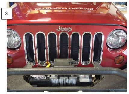
Install the remaining six surrounds using the center surround as a guide. Be sure they are all aligned before pressing down to fully seat the adhesive tape.
