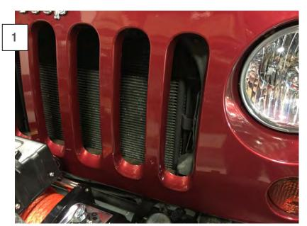
Begin by thoroughly wiping down the area of the grille where the inserts will adhere. Be sure the grille area is clean and free of any grease, dirt, or dust.
