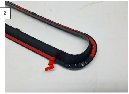
Peel the backing from the 3M tape on the grille insert and install in the center grille opening.
