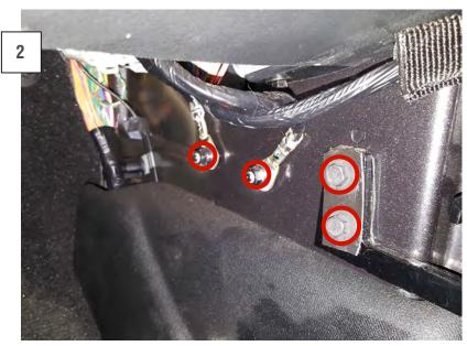
Remove the (2) 10mm door strap hook bolts and strap hook. Then remove the (2) 10mm electrical ground nuts.
