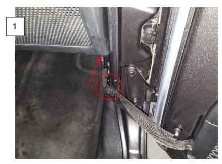
Begin by disconnecting the door's electrical connection. Follow the door strap under the dash to locate the plug. Once the plug is disconnected, unhook the door strap from the vehicle.
