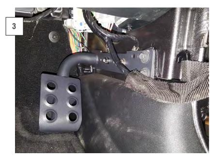
Install and secure the dead pedal using the factory hardware. Then reconnect the door's electrical connection, and door strap.
