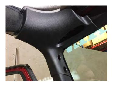
**Step 3\\** Remove the upper trim panel, pull the panel down away from the body of the vehicle.
