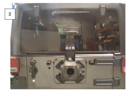
Install the (4) factory screws to the new third brake light.
