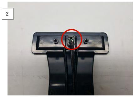
Plug the third brake light harness into the new third brake light.
