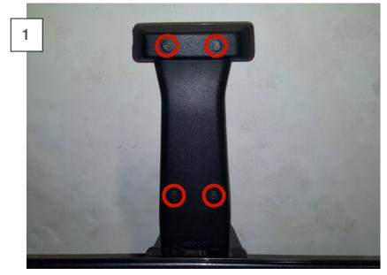
Begin by removing the (4) screws that hold the factory third brake light to the tire carrier. Unplug the wiring harness from the third brake light and remove the third brake light from the vehicle.
