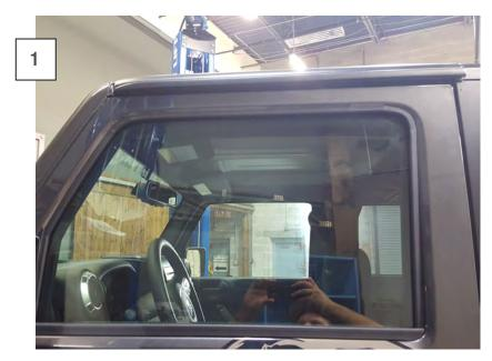
Begin by thoroughly wiping down the area of the doors where the rain guards will adhere. Be sure the door area is clean and free of any grease, dirt, or dust.
