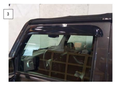
Install the remaining rain guards. Be sure they are all aligned before pressing down to fully seat the adhesive tape.
