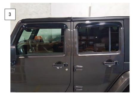
Install the remaining rain guards. Be sure they are all aligned before pressing down to fully seat the adhesive tape.
