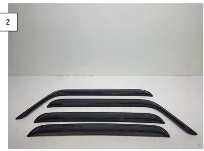
Peel the backing from the 3M tape on the rain guards and install on the top edge of the doors.
