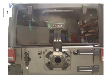
Begin by removing the spare tire from the vehicle.
