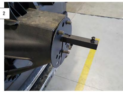
Line up the holes, and slide the license plate holder onto the threads of the spare tire carrier. \*\*Spare tire will keep this from coming off.
