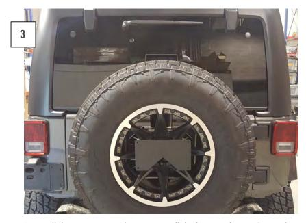
Reinstall the spare tire, and secure. Install the license plate end onto the shaft coming through the spare tire and tighten the allen bolt to secure.
