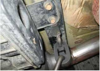
**Step 8:** Slide the supplied assembly bracket over the aFe Muffler Pipe (The hanger rod should face the bottom and point left), (x1) supplied 2.5" band clamp and install onto the y-pipe, the rubber hanger mount and the new installed aFe hanger bracket.
