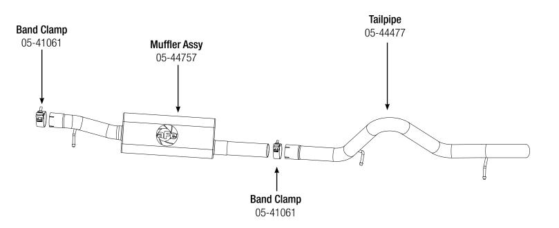
**Step 1:** (Read Instructions prior to installation) Remove your stock exhaust from the rear of your truck working your way forward. Take caution not to damage the factory isolation mounts as they will be reused. It may be helpful to lubricate the isolation mounts prior to disassembly. It is recommended to not fully tighten the clamps until the entire system has been installed.
