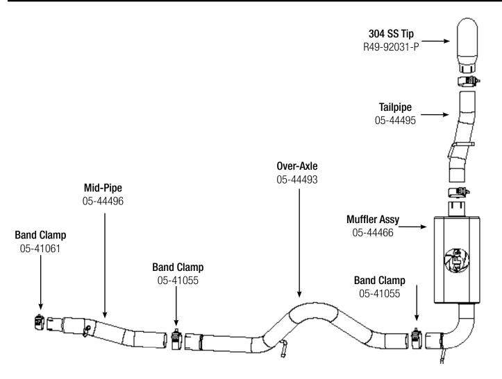
**Step 1:** (Read Instructions prior to installation) Remove your stock exhaust from the rear of your truck working your way forward. Take caution not to damage the factory isolation mounts as they will be reused. It may be helpful to lubricate the isolation mounts prior to disassembly. It is recommended to not fully tighten the clamps until the entire system has been installed.
