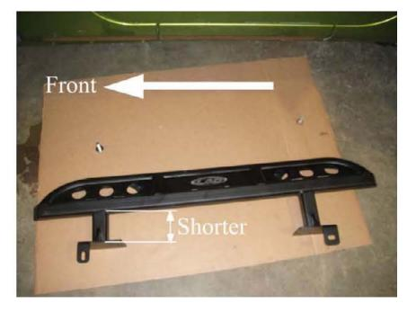
6. Using the factory hardware, secure your new LoD Signature Series Rock Slider to the points where the automatic transmisson and transfer case skid plates attach the frame rail on your Jeep JK Wrangler. An 18mm socket will be needed for this job. (Note: If your jeep has a manual transmission you will need spacers to make up thickness of this cross-member. If no spacers are used the sliders will not follow the body line.)
