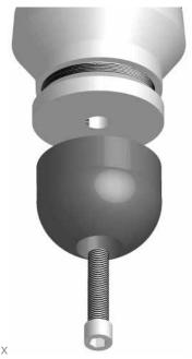
O Secure the Polyurethane Bump Stop (G) to the Bump Stop Plug (F) by installing the 3/8" Flat Washer (I) and 10mm Locking Nut (J) from above the upper spring mount.
