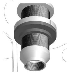
O Install Bump Stop Adapter (E) onto Threaded Tube (A) and tighten by hand until snug.
