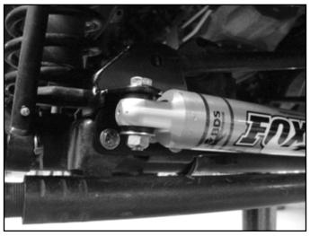
If using the factory steering stabilizer, use the factory axle hardware to mount it to the bracket. If an aftermarket stabilizer is installed, use the provided 1/2" bolt, nut, and washers from bolt pack J110. The larger diameter washer is used on the bottom against the stabilizer bushing.
