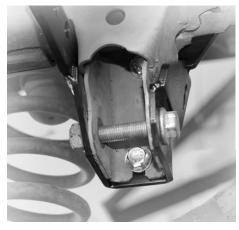
O Tighten all four (4) steering box bolts to 70 ftlbs. using a torque wrench. Product: Sector Shaft Brace
