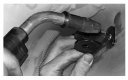
O Fuse the Frame Bracket (P) to chassis by plug welding each side of the mounting flange.
