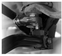
O Lower vehicle to ground and tighten track bar bolt to 125 ft-lbs.
