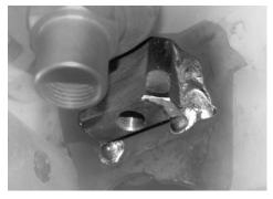
O Bottom of Frame Mount may also be welded to chassis as long as bead does not interfere with re-installation of Pillow Block. *HINT:* Edges of weld-on mount and Pillow Block are chamfered to provide clearance for small weld bead.
