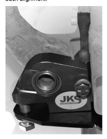
Once Steering Sector Pillow Block (E) is properly positioned, add tension to both 3/8" x 1" Bolts (L) and 1/2" x 2" Bolt (U) until snug to prevent Pillow Block from accidentally moving.
