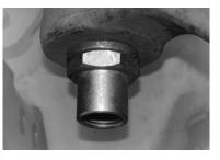
O Loosely install Pillow Block Frame Mount (I) on Steering Sector Pillow Block (E) with the 7/16" x 1-3/4" Bolt (J) and 7/16" Split Washer (K) exactly as illustrated below.
