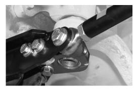
HINT: The extra 1/2" Locking Nut (W) & 1/2" Flat Washer (V) supplied with Front Trackbar Chassis Brace are not used when mounting to Steering Sector Pillow Block (E).
