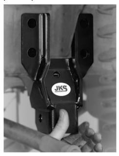
Re-insert the original steering box bolts and thread into mounting holes by hand. Do not tighten yet.  Insert OE track bar bolt (to keep mounting holes aligned) and loosely install original nut. Do not tighten.
