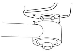
IMPORTANT: The Chassis End of Adjustable Trackbar must be in the "neutral" position (as illustrated above) before the Jam Nut is tightened.
