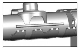
*HINT*: A die grinder with sanding wheel or similar tool is useful for removing paint from axle housing. This step may be easier with the Trackbar Brace temporarily removed.
