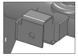
• Slide Trackbar Brace over factory track bar bracket as illustrated below. Make sure hole in Trackbar Brace aligns with bolt hole in factory track bar bracket.
