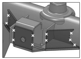
• The indicated locations on back side of axle must also be prepared for welding.
