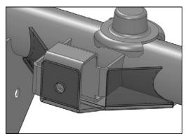
**HINT**: The snug fit should hold the brace in position for welding.
