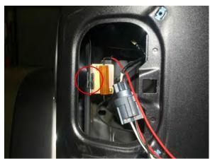
Step 5: Reconnect the vehicle's chassis harness to Raxiom tail light. Ensure the circled tabs are located behind the vehicle's sheet metal before installing the factory screw. Reconnect the battery terminal and ensure the tail light
