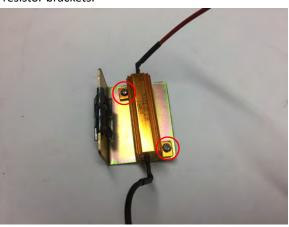
Step 4: Press the resistor mounting bracket onto the sheet metal.
