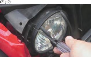
**Step(7)** Repeat steps 5 and 6 for the installation of the other Euro Guard lamp retainer ring.
