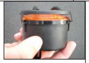
**Step 5.** Slide the remaining guard tabs onto the housing. The fit will be tight.
