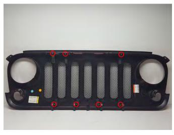
**Step 3\\**Fasten the grille overlay to the factory grille using the (7) M4 bolts and nuts.
