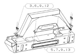
2. Install the wing, and install the bumper to the vehicle.
