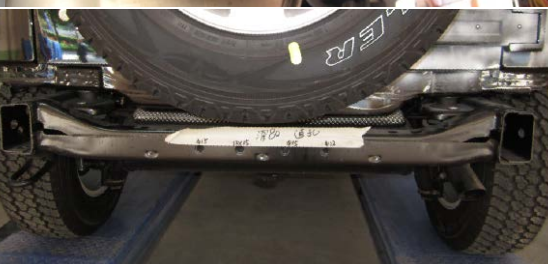
Bolts holding the crash bar
