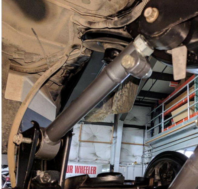
Figure 3. Installed Upper Control Arm
