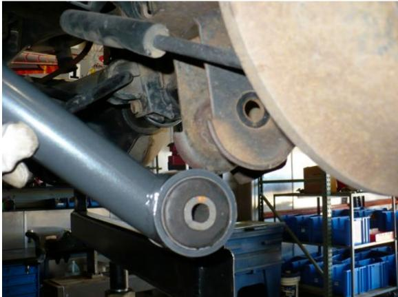
3. Tighten the factory control arm bolts to 125 ft-lbs, wait until the vehicle is at ride height before tightening the bolts as to prevent preloading the control arm bushings.
