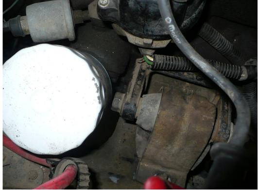
9) Remove the attachment bolts at the block and remove the assembly. Retain all OEM hardware for motor bracket.
