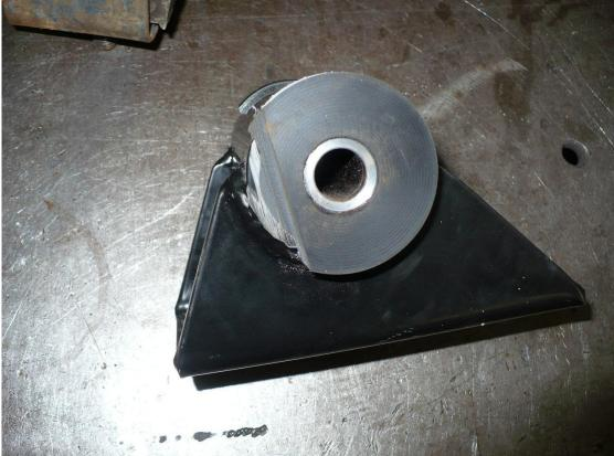
5) Install the 8251 motor mount as shown below. Use the OEM through bolt / hardware. Use the factory bolt for the threaded hole at the outer attachment point and use the 3/8-16 UNC x 1.0" long bolt provided for the inner attachment point. Use a washer under both the bolt head and corresponding stover nut for the inner attachment point.
