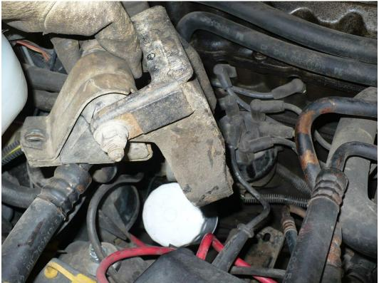
10) With bracket removed from vehicle, replace the factory motor mount with the 825101 motor mount.
