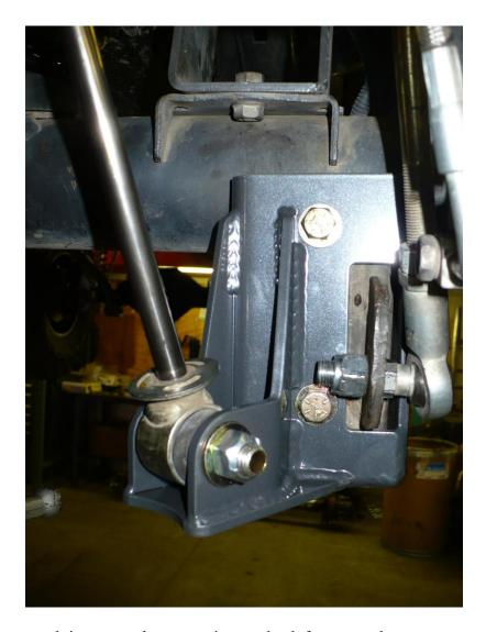
13) Note, now is a good time to cycle suspension to check for proper bump-stop spacing to ensure shock does not act as bump stop. Use the approximate collapsed shock measurements below as a reference.
