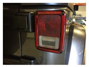
**Step 2:** Disconnect the tail light plug and then remove the light from the vehicle.
