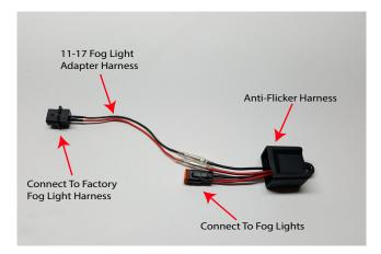
STEP 8 // Connect the anti-flicker harness to the fog light adapter harness. Connect the fog light adapter harnesses to the factory fog light wiring harnesses. Connect the fog light to the anti-flicker harness. \*\*Note: There are (2) different style factory fog light connectors. Use the correct harness for your vehicle.
