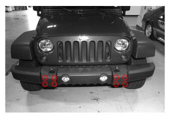
STEP 3 // From under the vehicle, access and remove the (8) 18mm nuts securing the factory bumper to the vehicle.
