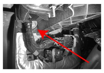
STEP 12 // Optional Light bar Wiring: Route the on/off switch to the interior of the vehicle. Mount the switch in the desired location. Zip tie any extra loose wiring out of the way.
