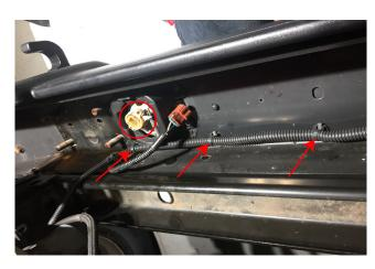
STEP 2 // From under the vehicle, remove the factory fog light connectors and free the fog light wiring loom from the bumper.
