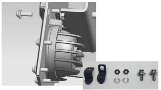
STEP 6 // Insert the (1) M6 bolt through the empty hole in the fog light bezel plate. Attach the fog light hook clip around the fog light, and secure it in place with (1) M6 hex nut, and flat washer. Repeat the process on both sides.
