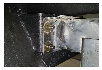
STEP 7 // Install the bumper by using the (4) M10 nuts, (4) M10 x 25mm bolts, (8) lock washers, and (8) flat washers to the vehicle. Torque to 40 lb ft.
