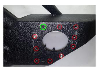
STEP 4 // Install the fog light bezels to the bumper by using the (18) M6x1.0x20mm Bolts, lock washers, and flat washers. \*\*Note: Leave the hole highlighted in green empty until step 6.
