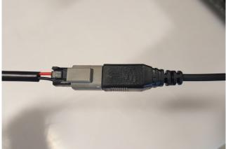
STEP 10 // Optional Light Bar Wiring: Connect the light bar into the supplied harness. Zip tie any excess wire away from moving and/or hot engine components.
