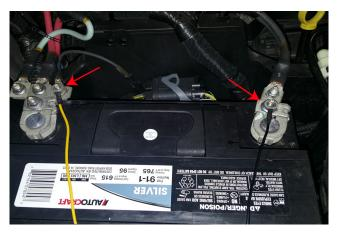
STEP 11 // Optional Light Bar Wiring: Install the yellow 12+ volt wire to the positive battery terminal. Connect the black ground wire to the negative battery terminal. Secure any extra wire out of the way.
