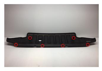
STEP 1 // Remove the (6) plastic push pins securing the factory splash shield to the vehicle. (4) Across the front edge, (2) on the rear edge.
