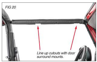
**Step 8: For all 97-02 TJ Wrangler Vehicles** Installing over Door Horizontal tubes. Place a fabric covered foam tube onto each of the horizontal bars.
