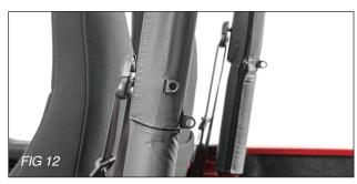
For soft top models, slip the pre-cut (step three) openings over the pivot bracket on each side of the vehicle. See Fig 12.
