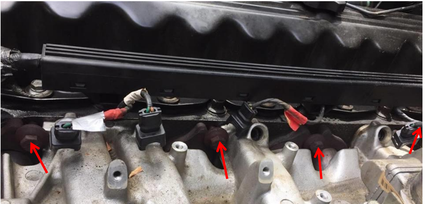
23. Remove bolts holding intake/exhaust manifold, using a 9/16" box end wrench. There are 4 bolts on top and 4 on the bottom and also 2 nuts on the bottom.
