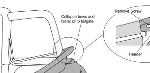
Manufacturing Note: Due to a recent header assembly modification by Daimler Chrysler, the plastic strip on the windshield header may have 8 screw locations instead of 14. Both attachment numbers of screws will securely fasten the header and perform as the original design was intended.
